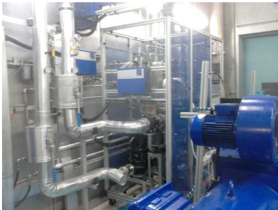
Figure 4: Thermal shock rig (test cell side) with test bed (blue), routing valves and pipes on the left.
