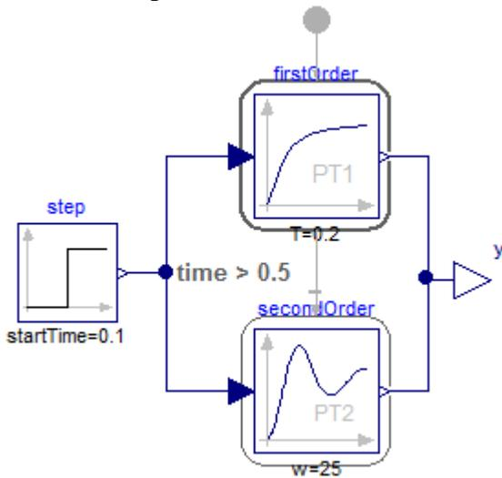
Figure 10: State machine switching between two input-output blocks.
