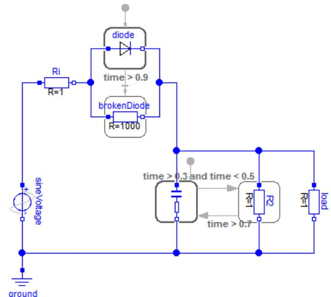
Figure 5: Circuit with two acausal state machines.
