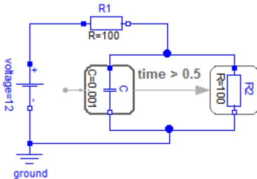
Figure 7: Simple circuit with an acausal state machine.
