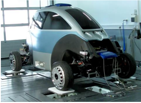
Figure 7: ROMO on the four-post test rig
